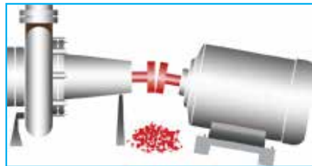
Fig 5.2.3 : Effects of misalignment
