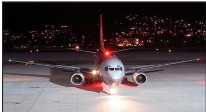
Fig 3.1.1 (b) Anti-collision Beacon Lights
